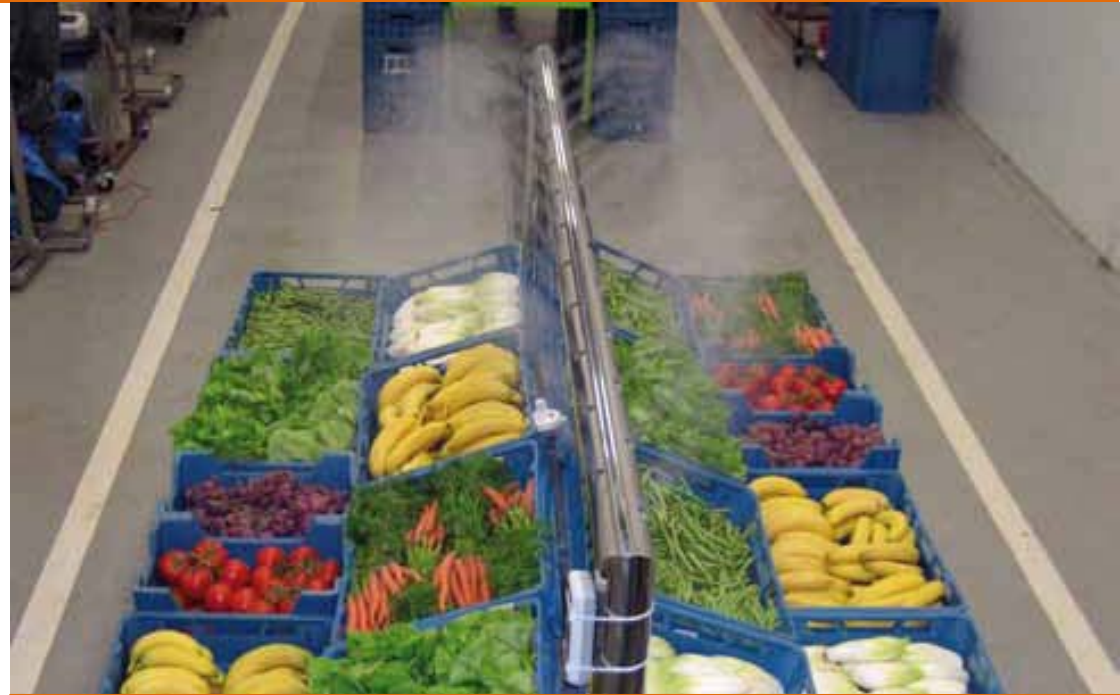
Trial arrangement for research into the conserving effect of spray
