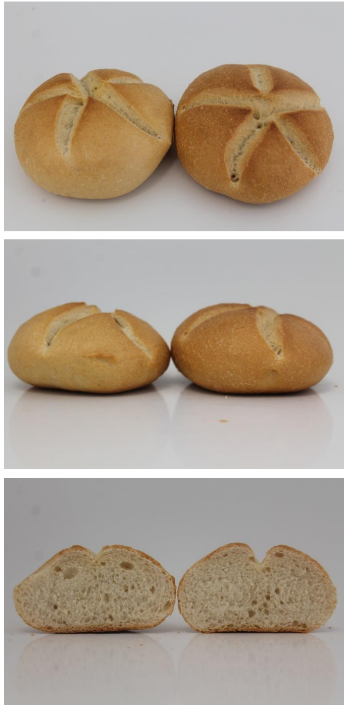
Figure 16: Comparison of direct proofed products at 35°C and a relative humidity of 80% with ultrasonic humidification(left) and conventional electrical humidification (right)
