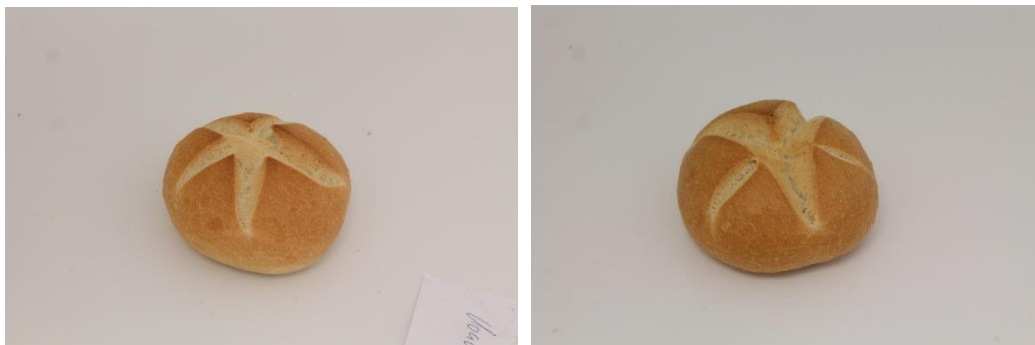
Figure 5: Comparison of the products proofed with electrical humidification (left) and ultrasonic humidification (right) in the direct proofing process
