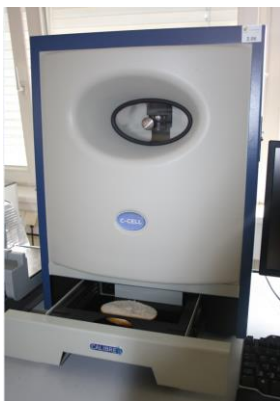
Figure 1: CCell from Calibre (above is the camera and below a drawer in which the product is placed)
