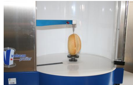
Figure 3: VolScan with clamped roll. The laser scan drives round the product to detect the volume
